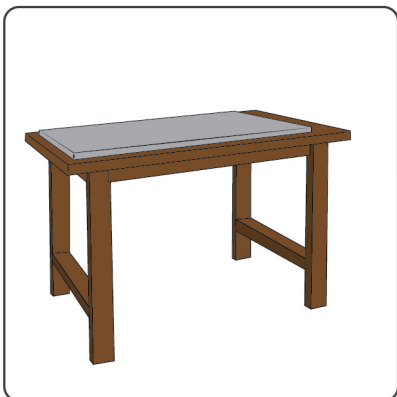
Stable Work Table With Sacrificial Board/Fibre Cement
